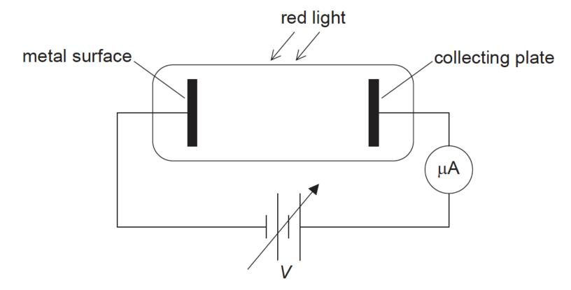
The potential *V* of the supply is varied and the current is measured. The results are shown on the graph.
