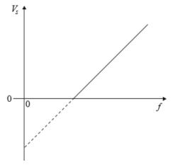
Planck's constant may be determined from the charge of an electron  $\boldsymbol{e}$  multiplied by
